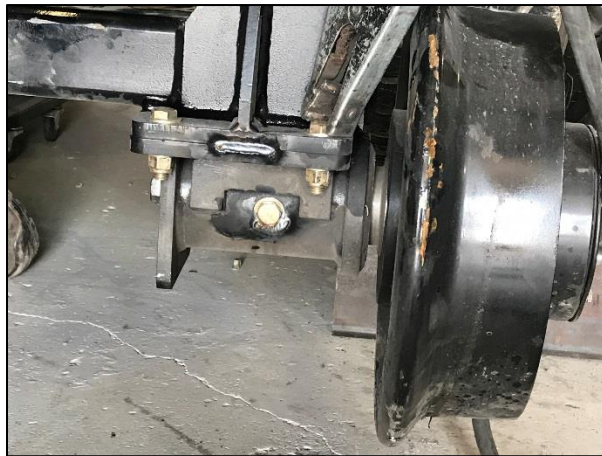
Figure 14: Welded Spindle Housing (Toe and Gauge Adjustment Locked)
